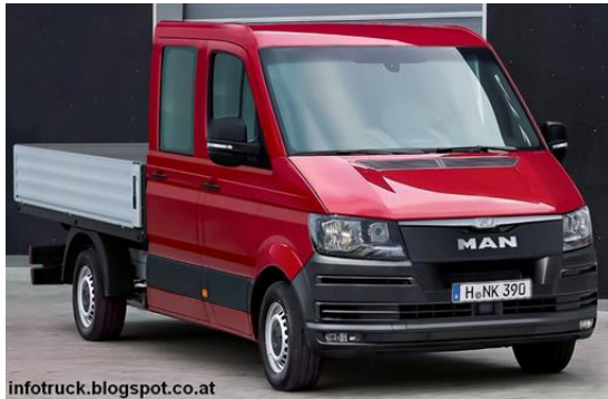
Figure 46: Example for a light truck with a GVWR of 5.50 t
