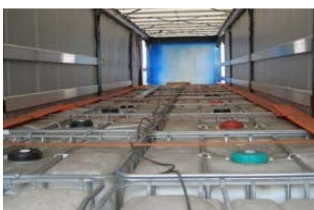
Figure 38: Water tanks in the trailer of HDV 4
